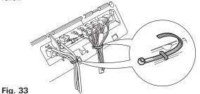
All cables must be securely attached and must not become loose or disconnected due to vibration – risk of fire!
